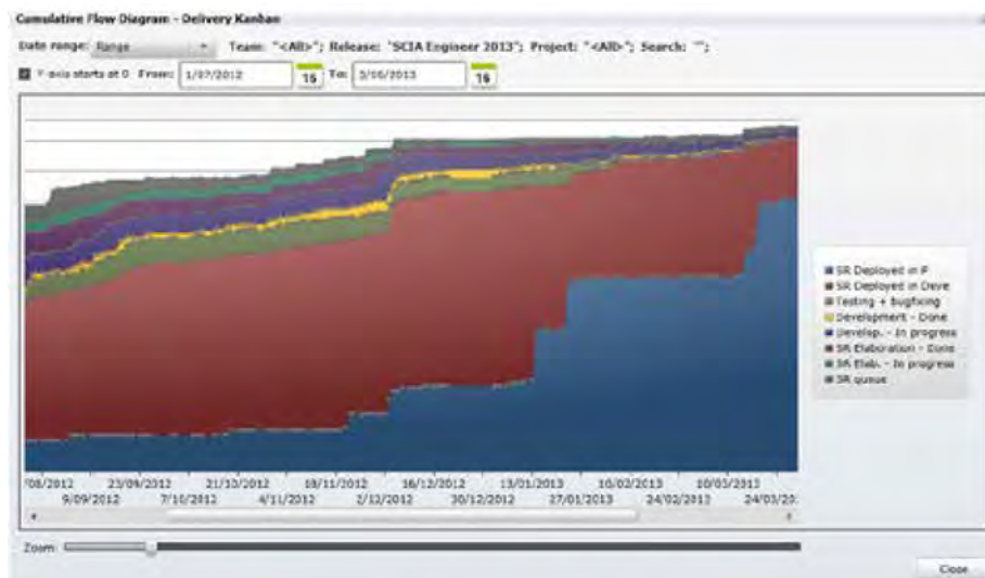
Figure 1.4 An example of a cumulative flow diagram that can be generated from the Kanban system. The unevenly rising red part represents the distribution of work that has been performed for the merging of a feature into the larger product. The merging has not been happening concurrently with the delivery but rather in large chunks, and only when it was critical.
